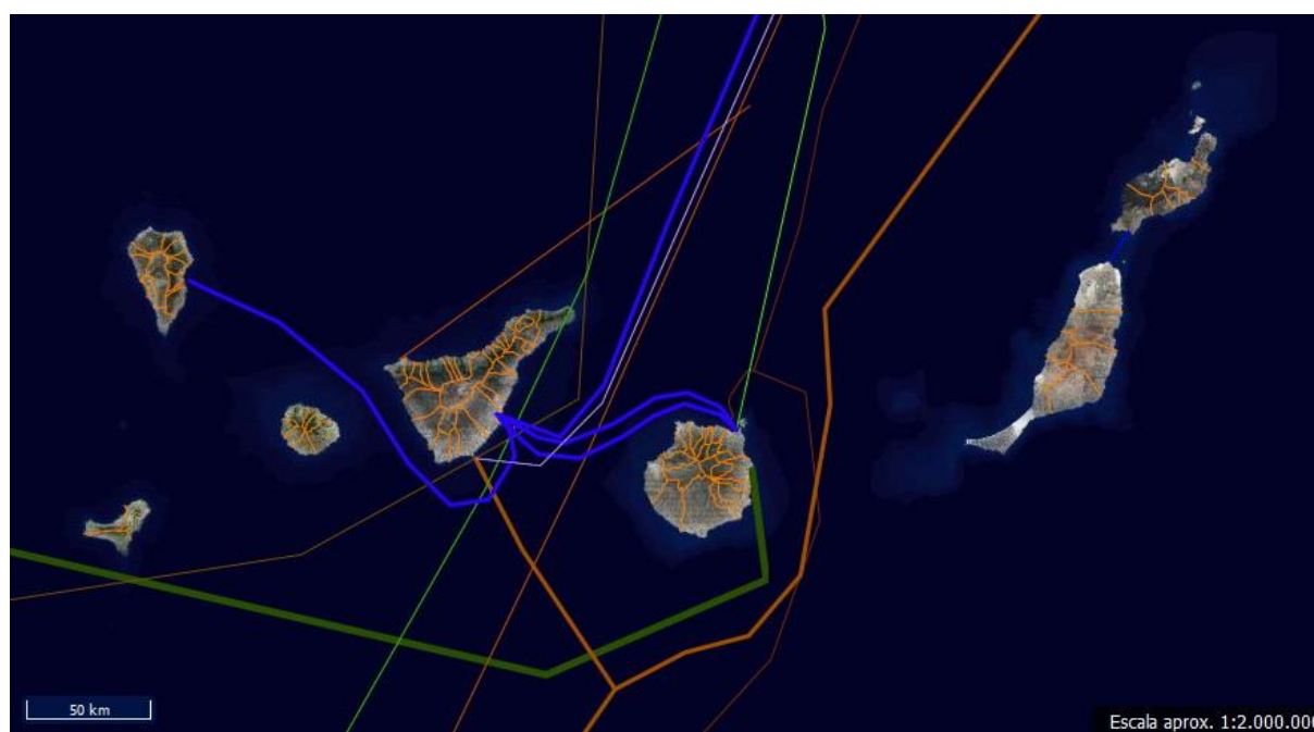
Figure 273. Telecommunication cables (source: cablemap.info) and electric cable (source: viewer HPL, 2019).
