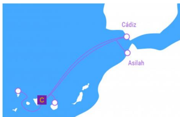
Figure 272. Canalink cable system showing the connections inter-islands and with Morocco ( http://canalink.iter.es/ )
